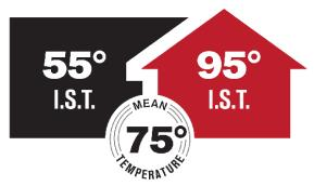
75°F mean reference testing temperature with a 40°F differential **I.S.T. represents the temperature of the two defined outer most insulation surfaces**
